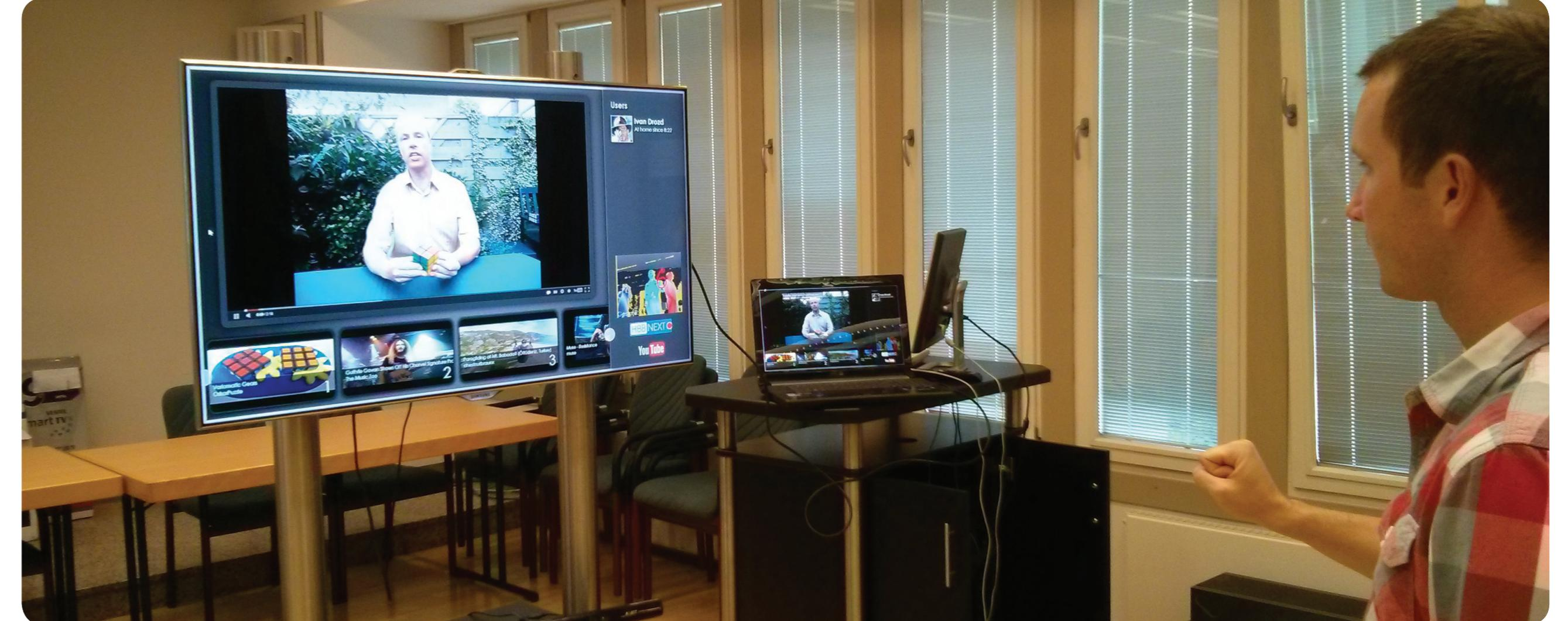
We have created an application demonstrating the gesture recognition-based control of the video player. The Kinect sensor allows to capture static and dynamic gestures which are processed by our in-house algorithms. Based on the YouTube API, the application allows to command the player as well as browse through the video recommendations provided by the well-known service. The user-friendly environment
